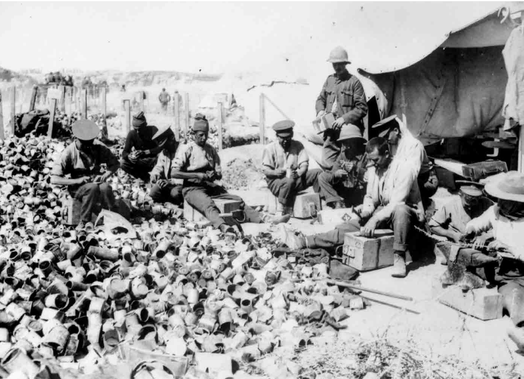
Men assemble jam tin bombs near the beach at Anzac Cove. At Gallipoli the Anzacs, chronically short of purpose-made grenades (bombs), made crude versions from old tin cans filled with fragments of Turkish shells and barbed wire cut into short lengths. (AWM H10291)
