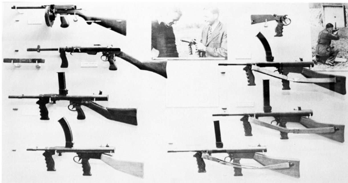
Owen Gun Prototypes & Experimentals. On display at the Australian War Memorial, Canberra Left side, from top— .22 RF, 1939; .32 ACP, 1941; .45 ACP, 1941; .380 revolver, 1941. Right side, from top— Mk I action; .380 revolver, trials, 1941; .45 ACP, trials, 1941; 9mm Para., trials 1941.
